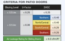
The ENERGY STAR program for windows divides the country into four distinct climate zones to recognize the varying heating and cooling months among the states. For patio doors, there is only one U-Factor and one Solar Heat Gain Coefficient (SHGC) requirement for ENERGY STAR compliance.
